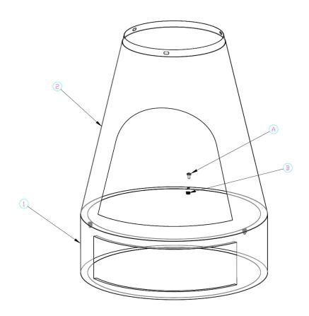
**Step 2**: Assemble the Shoulder Body (3) to the connected Fire Body with Screw (A) and Nut (B), than Fix them
